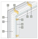
01. Render 02. Fiber cement board 03. Nailing batten 04. Gypsum wallboard 05. Insulation 06. Vertical stud 07. Plastic foil 08. Insulation 09. Horizontal stud 10. Gypsum wallboard
