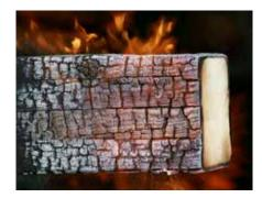
Wood burns in a controlled manner and a cross section can be chosen so that the beam can bear the required load.
