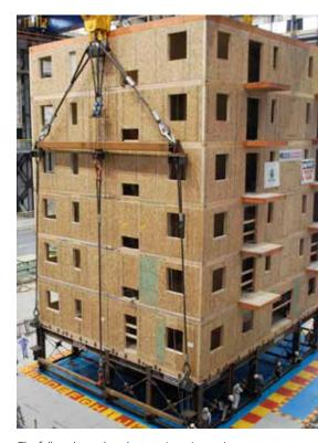
The full-scale earthquake test. Japan's massive E-Defense Shake Table, the largest shake table in the world
