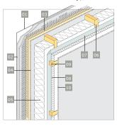
01. Finishing render 02. Render with reinforcement net 03. Insulation 04. Gypsum wallboard 05. Insulation 06. Vertical stud 07. Plastic foil 08. Insulation 09. Horizontal stud 10. Gypsum wallboard
