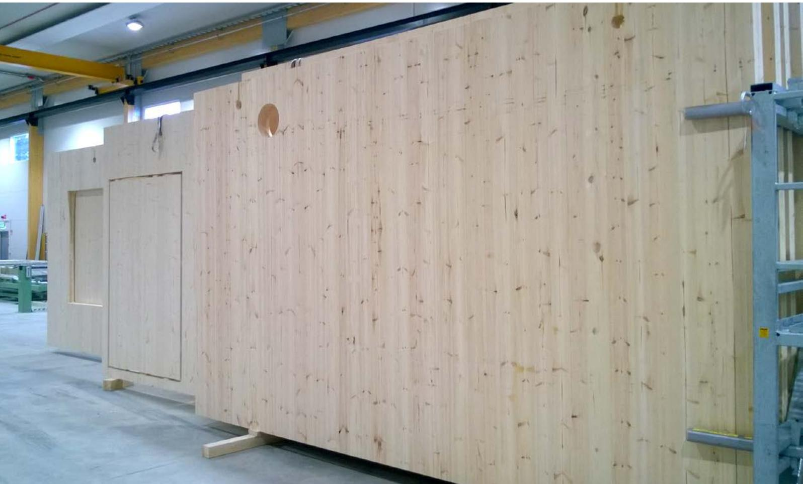
CLT panels ready for wrapping and delivery.
