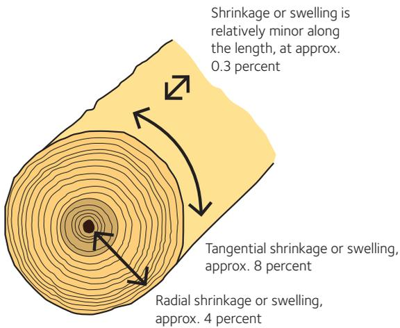
**Figure 2** Shrinkage or swelling in a softwood log from fresh to fully dry. Shrinkage or swelling in a piece of timber varies depending on how the growth rings are positioned in the wood. The smallest dimensional changes occur in wood where the growth rings are perpendicular with the face, known as vertical grain.
