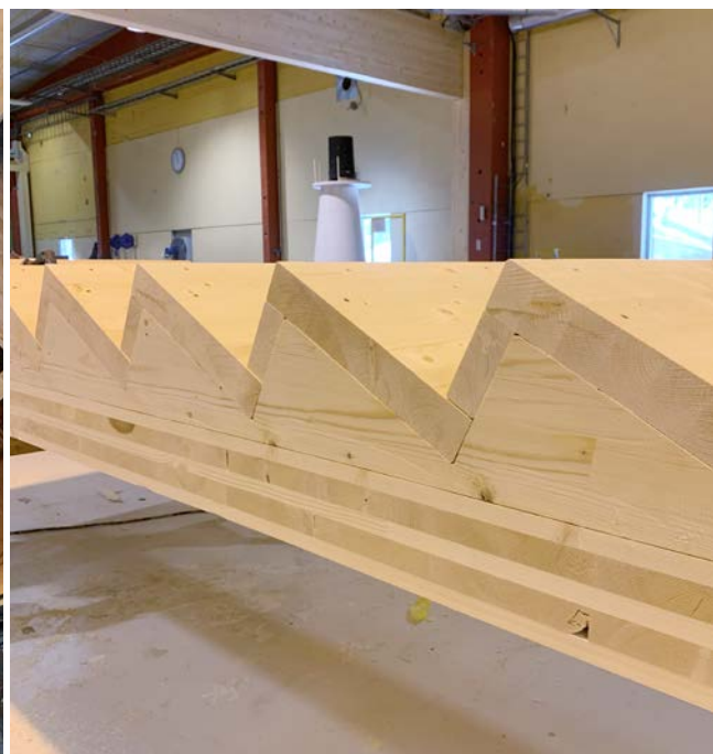
Stair carcass in CLT.
