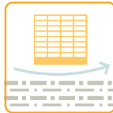
Use supports and make sure the ground is drained
