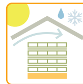
Treated wood should be protected under a top cover
