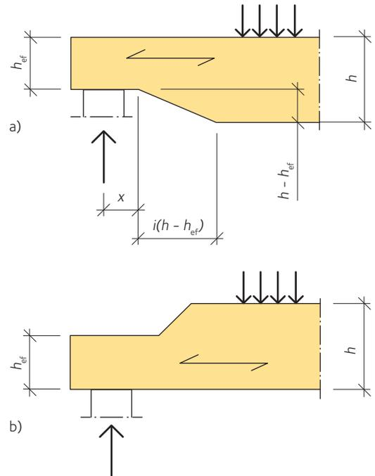
Figure 8.3 End-notched beams
