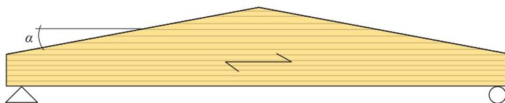
Figure 8.1 Double tapered beam
