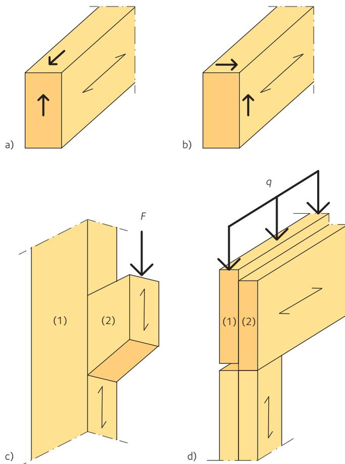
**Figure 3.1** a) Member with a shear stress component perpendicular to grain (shear).
