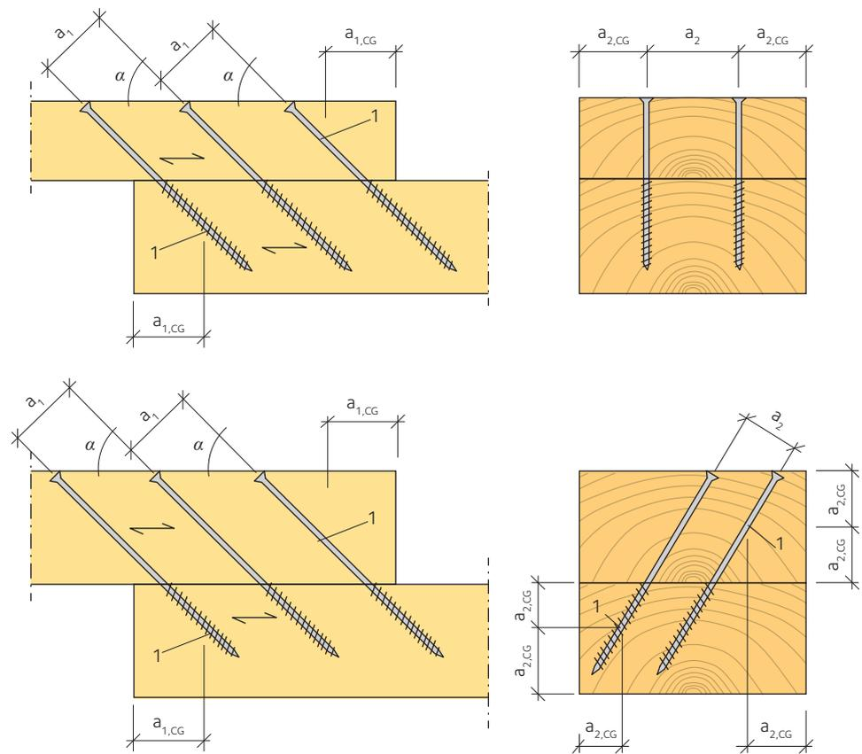
**Figure 10.6** Spacing and end/edge distances for axially loaded screw connections
