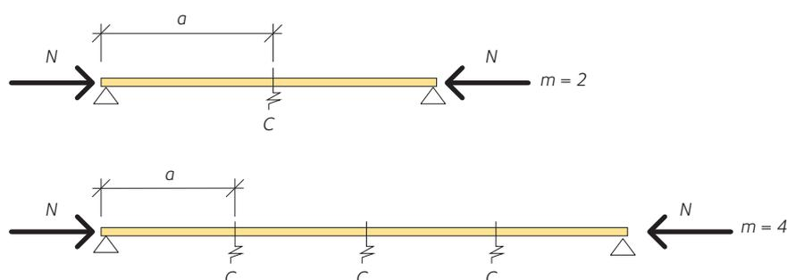
Figure 12.1 Single members in compression braced by lateral supports (C)
