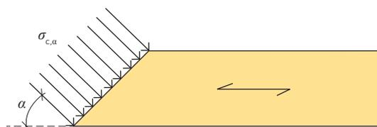
Figure 7.1 Compressive stresses at an angle to the grain
