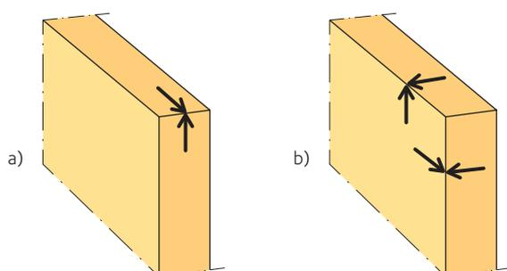
**Figure 3.2** Definition of a) panel shear and b) planar shear.
