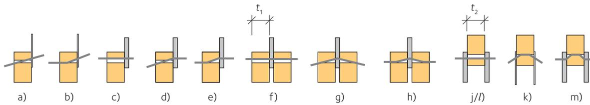
**Figure 10.2** Failure modes for steel-to-timber connections. The letters refer to the respective design expression above.
