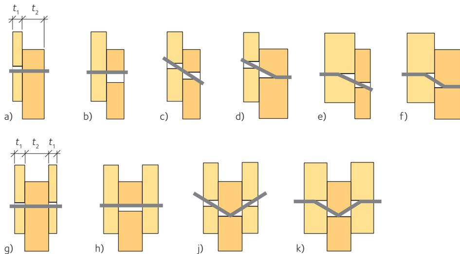
**Figure 10.1** Failure modes for timber and panel connections
