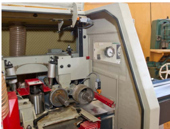
Safety switch stops dangerous moving parts when you open hatches.
