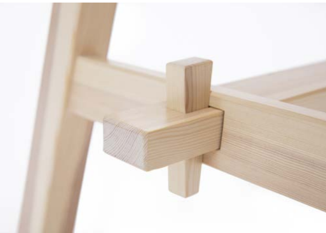
A keyed mortise and tenon joint is good for easy assembly. In this case the tenon goes through the leg and is wedged on the outside.
