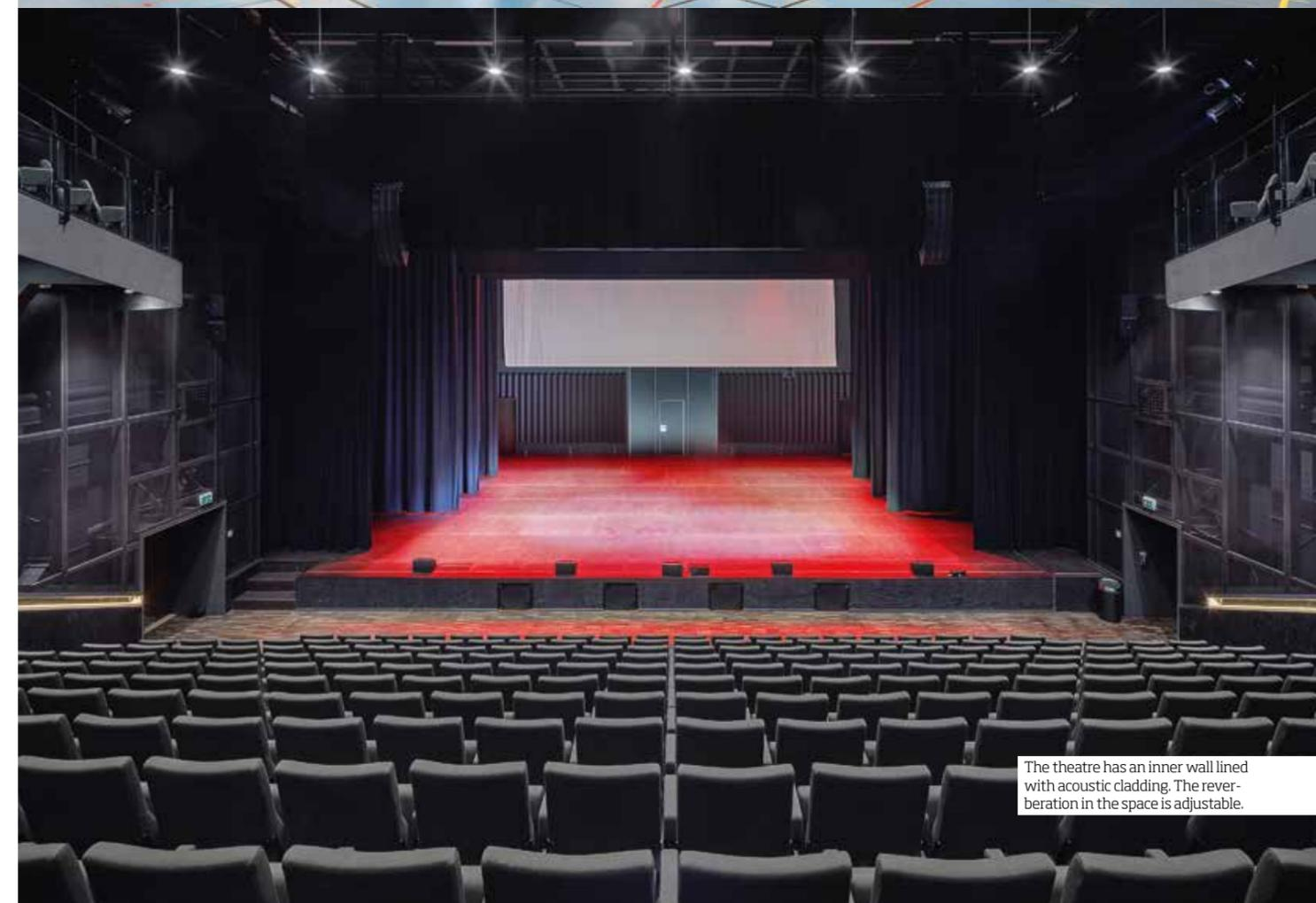
The theatre has an inner wall lined with acoustic cladding. The reverberation in the space is adjustable.
