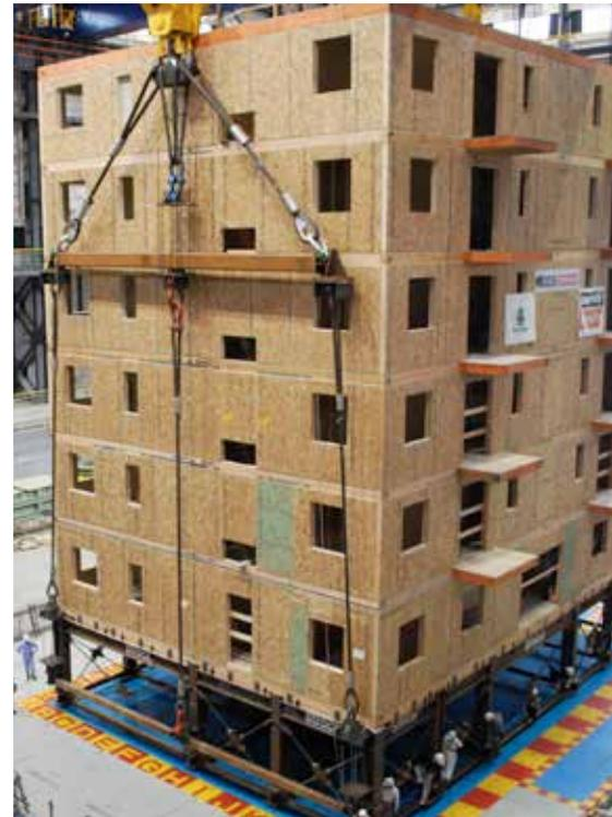
The full-scale earthquake test. Japan's massive E-Defense Shake Table, the largest shake table in the world
