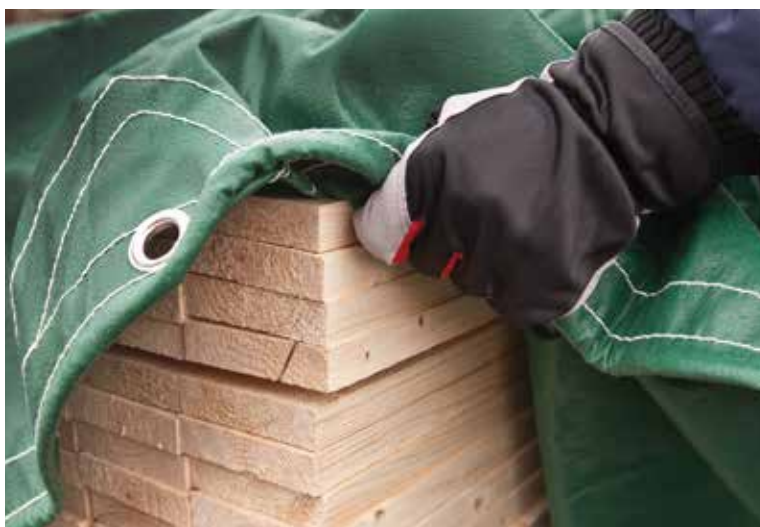
Keep glulam for outdoor use ventilated and protected
